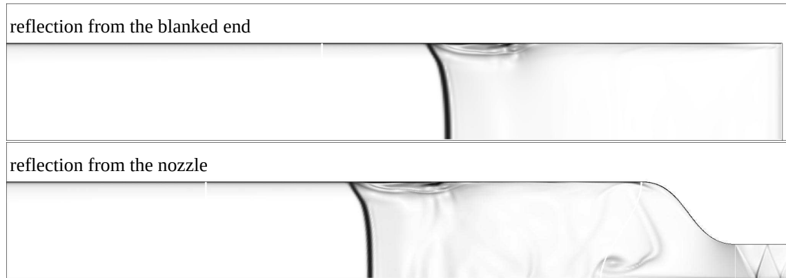
Figure 7.42: Comparison of numerical schlieren contour plots comparing the interaction of the reflected shock with the boundary layer following the reflection of the shock from the blanked shock tube end (top) and the nozzle (bottom)
