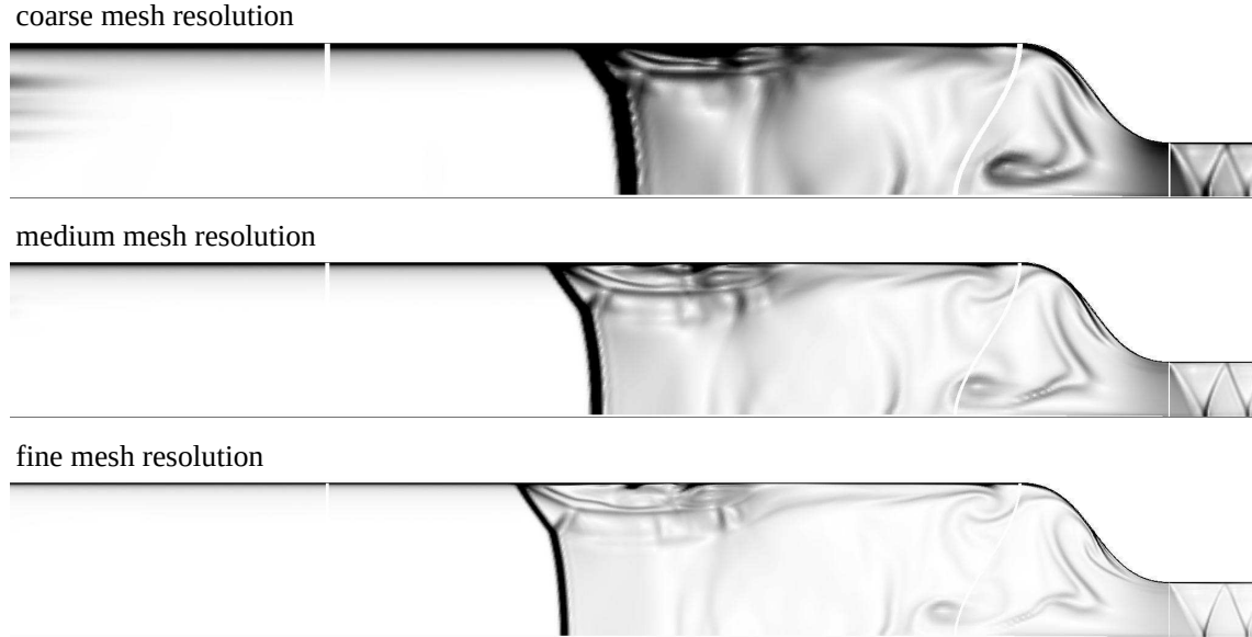
Figure 7.43: The effect of the mesh resolution on the modelling of the interaction of the reflected shock with the boundary layer. Numerical Schlieren images are shown, comparing the simulated flow for the coarse (top), medium (middle) and fine (bottom) meshes. The frames are shown at 300 \mu\text{s}
