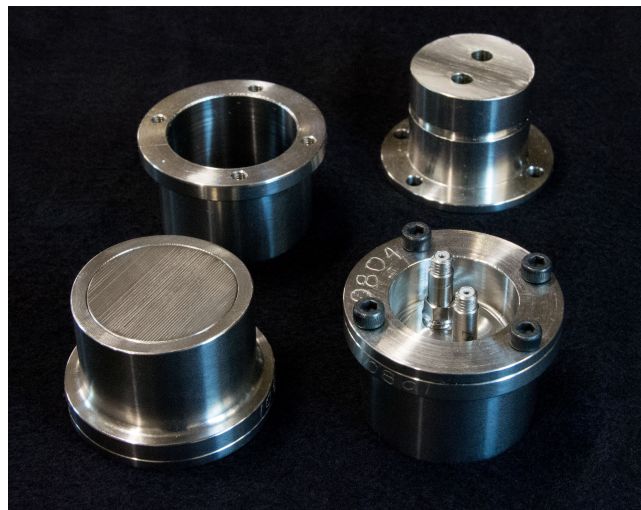
Figure 4.20: Nozzle wall sensors and optional plugs.
