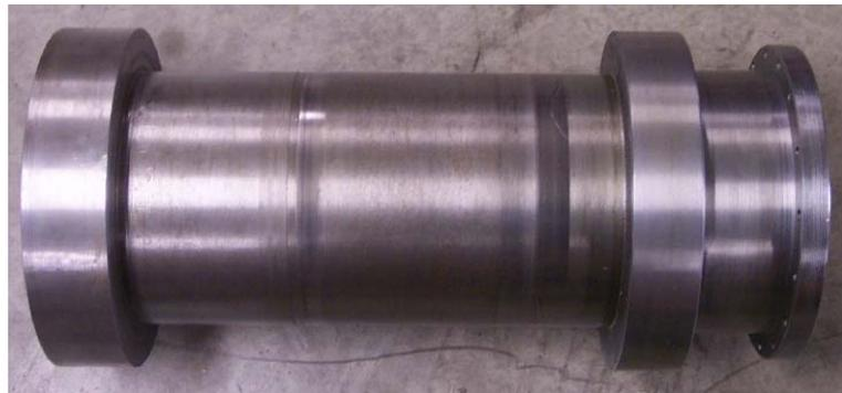
**Figure 5.7:** Section 2 of the nozzle before painting
