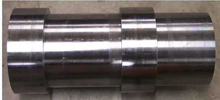
**Figure 5.8:** Section 3 of the nozzle before painting
