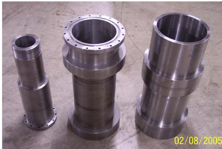
**Figure 5.9:** The 3 sections of the nozzle
