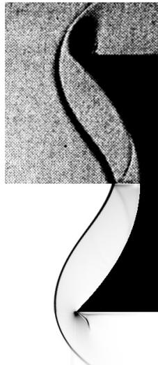
Figure 4.3: Focusing of a planar shock: Izumi et al. experimental Schlieren (top half), CFD-FASTRAN numerical Schlieren (bottom half).
