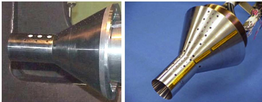
Figure 5.1: Hollow cylinder extended flare (HCEF) model.
