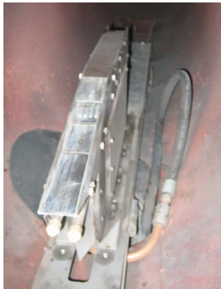
(b) picture of scramjet mounted in X2 dumptank on modified rail
