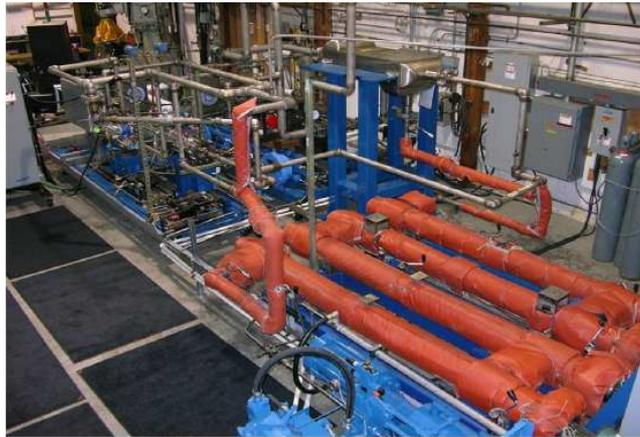
**Figure 2.5:** Photograph of the SNL sCO<sub>2</sub> Brayton loop [42].
