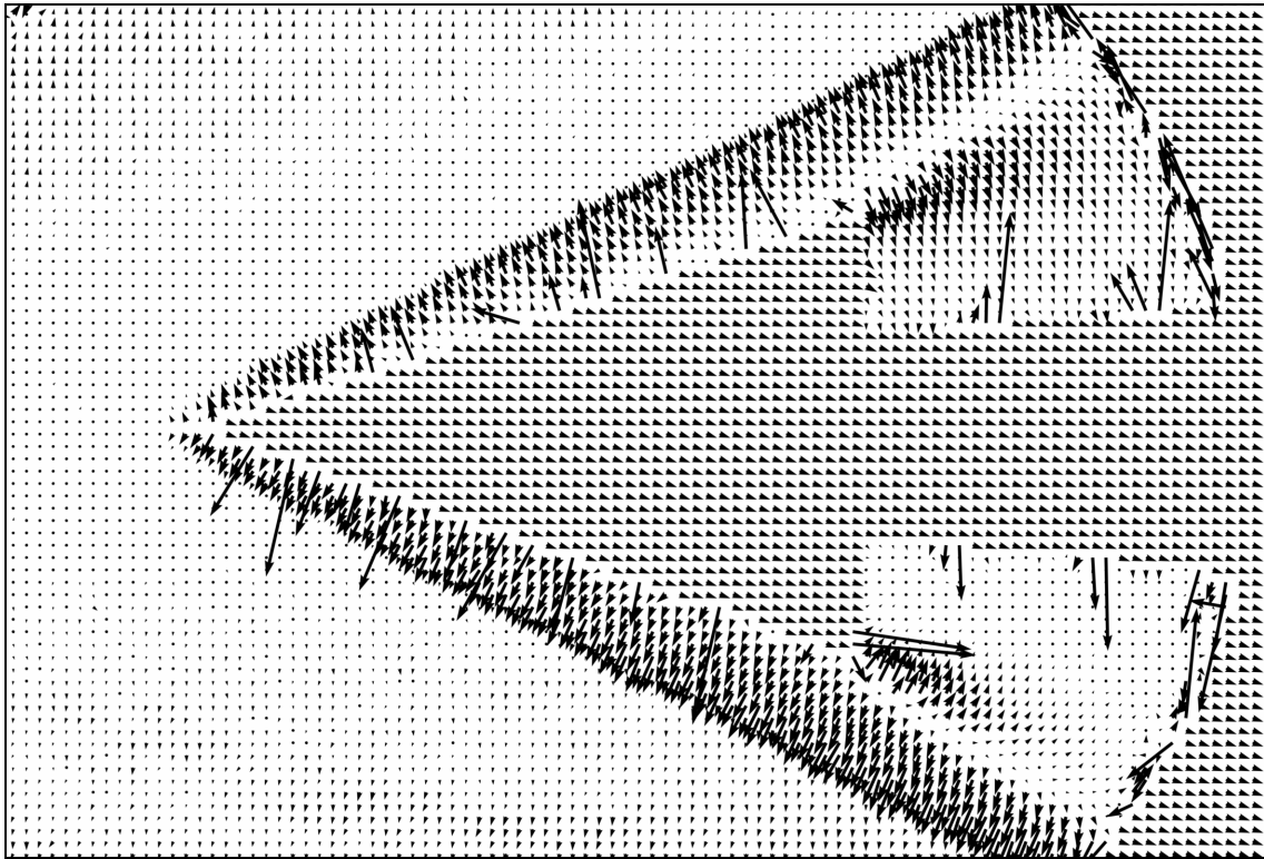
Fig. 5.9. Arrows showing density gradient vectors for a search window size= 32 x 32 and step size = 16 pixels.
