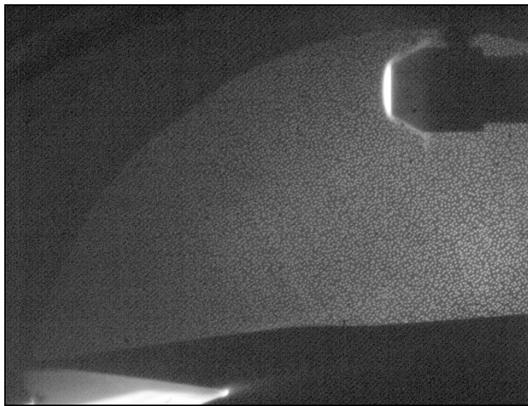
Fig.5.33. Shot 8772, p_s = 31.7 MPa, h_s = 6.0 MJ/kg, M_\infty = 7.2 , p_\infty = 2.9 kPa, U_\infty = 3.2 km/s, T_\infty = 505 K
