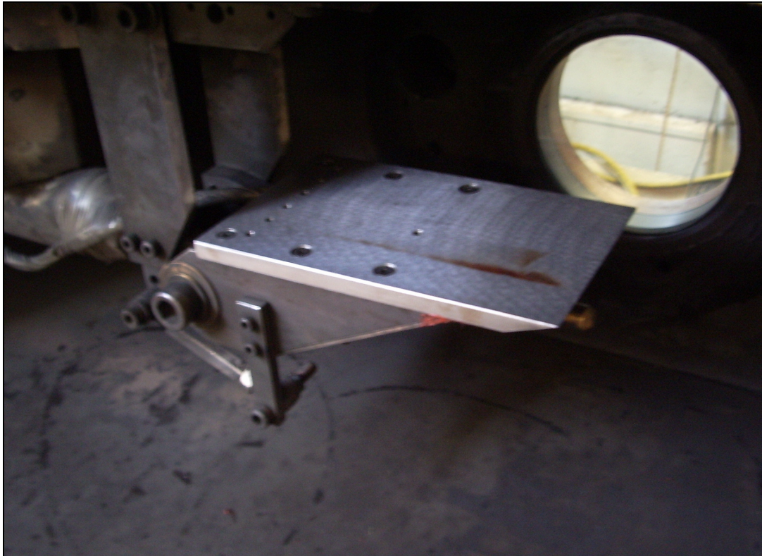
Fig.4.6. Flat plate mounted in T4 test section.
