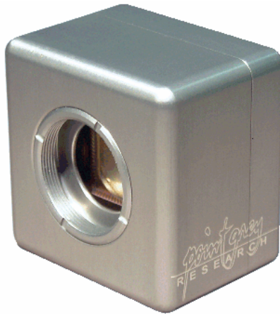
Fig.4.14. The Scorpion SCOR20S0 (Courtesy: Point Grey Research Inc.) Size: 50 mm X 50 mm X 40 mm Weight: 125 grams.
