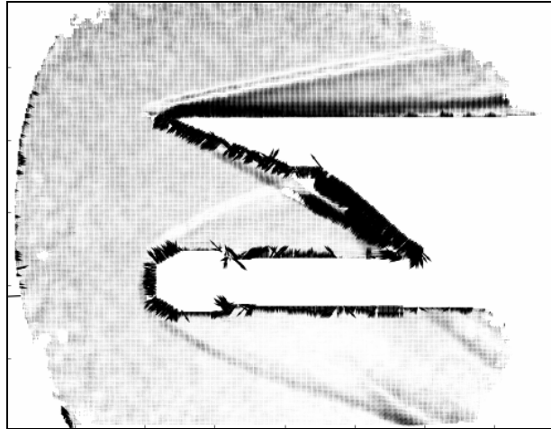
Fig. 5.39. Gradient vector image, shot 9058, search window size = 16 x 16 pixels, step size = 4 pixels.
