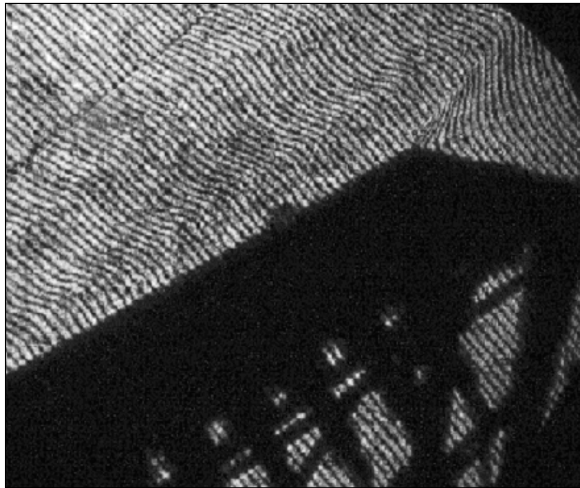
Fig. 5.49. Flow Hologram, shot 9167, p_s = 30.7 MPa, h_s = 4.3 MJ/kg, M_\infty = 7.3 , p_\infty = 2.6 kPa, U_\infty = 2.8 km/s, T_\infty = 363 K.
