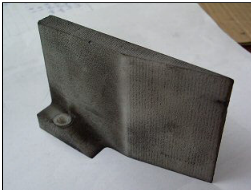
Fig. 4.7. SLS wedge to be mounted at trailing edge of the steel plate.
