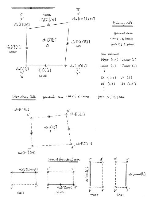
Figure 3: Cell, interface and vertex indexing in 2D for Eilmer3. The upper half of the figure shows the primary cells defining the finite-volumes for the conservation equations. The lower part of the figure shows the secondary cells, used for computing spatial derivatives.
