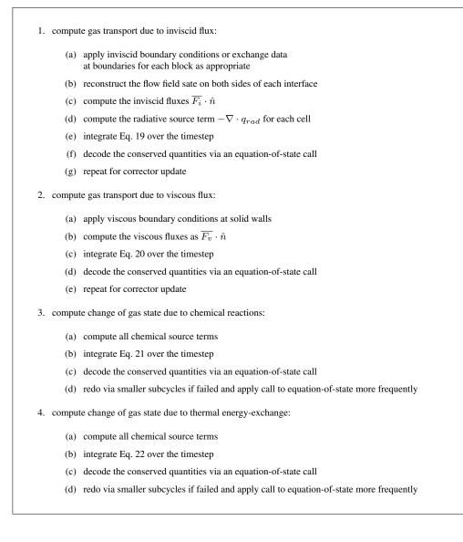
Figure 1: Sequence of operations for a time-step update in Eilmer3.
